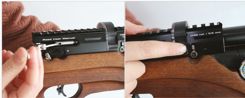
MAGAZINE Remove from right side the magazine that has run out of pellet will not permit new charge.
